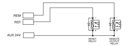
To protect the output stage, only 24V polarised relays with back EMF diodes should be used. If any of the relays are to be used to switch mains potentials, then suitable relays should be chosen and installed and wired accordingly, so as not to compromise the electrical safety of the fire alarm system.
