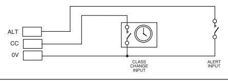
Connect the wiring for each input to the relevant 5mm connector block on the Main Control PCB and terminate their screens at the panel's base earth distribution post (see page 13 for more details).
