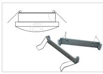
The semi - recessing kit for the Meteor LED includes retaining spring clips that fit securely to the luminaire. This allows the Meteor LED to become a semi - recessable fitting to the ceiling or wall.
