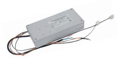
**SPECIFICATIONS Light Source** LED panel 26-55W **Emergency Duration** 3 hours (minimum) Mains Voltage 240V 50Hz ±10% Mains Current (max) 80-130mA **Recharge Period** Less than 24 hours Charge Indicator Integral green LED **Changeover Voltage** As per the requirements of BS EN 60598-2-22 **Temperature Range** Max 50° C 950g Weight Battery 2x 9.6V 1500mAH Ni-Cd
