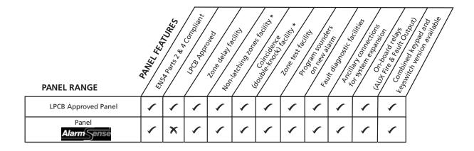
\* Non-EN54 Part 2 panel features: Coincidence Non-latching zones facility
